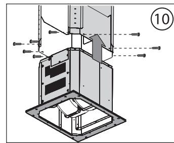
12. Extend upper duct cover to the ceiling and secure it to the duct cover ceiling bracket using the (4) screws previously removed when the assembly was taken out of the packaging. Fig. 12
