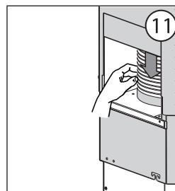
13. Lift the hood assembly into the top duct cover. Secure hood assembly to bottom support frame by using (4) screws. Fig. 13
