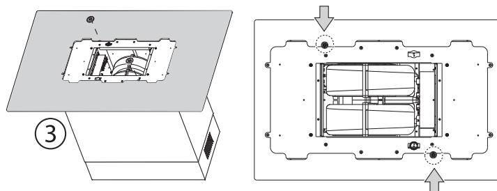
3. Take the lower duct cover from the duct cover extension kit and secure it to the hood assembly by following the instructions from step 2 in reverse order.
